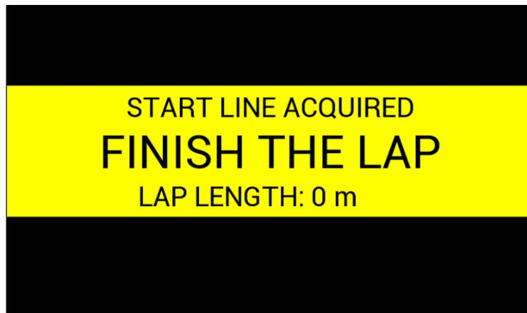
This overlay uses the channel `adu.track.userButtonDefinedTrackAcquiring` as a display condition. The ADU supports 3 types of the track definitions. The first one is the tracks defined in the device internal software (built in tracks), the second type is user track (5 available) that can be defined using the ADU software and the user tracks window. The third type is button defined track.
