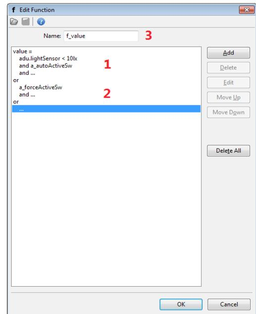
Now that the logic is done, assign the *Aux1* output so that it can be controlled with *f\_value*:
