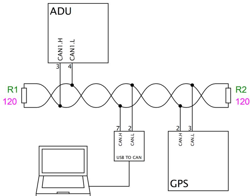
After wiring the GPS module, it is necessary to configure the ADU. In the CAN bus/Serial setup options, select the CAN bus that the GPS module is connected to (GPS, CANBus).
