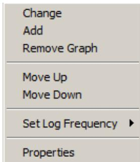
Here you can add a new log channel (**Add**), remove an existing log channel (**Remove Graph**), change a log channel (**Change**), or relocate a channel (**Move Up, Move Down**). You may also change the log frequency (**Set log frequency**) and change the display settings for a given channel (**Properties**).
