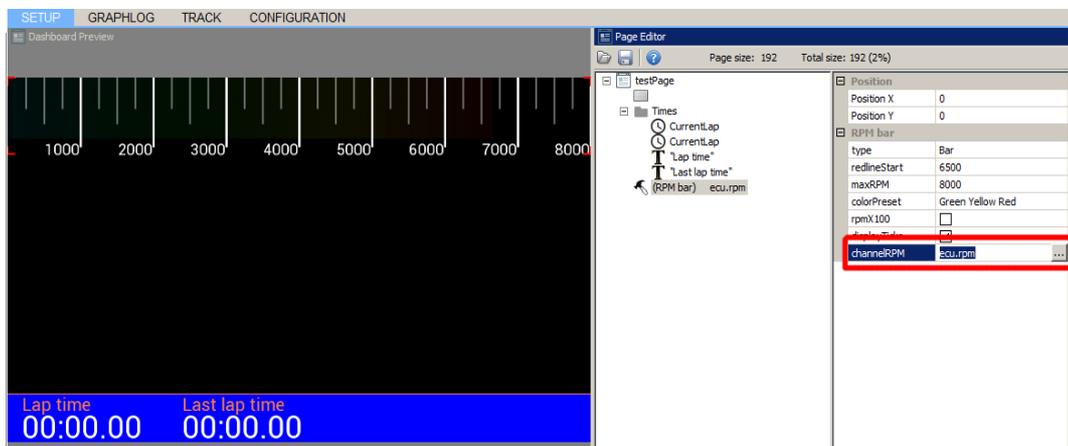
To test the operation of the indicator you can enter a numerical value (only integer values) in the **Channel** field. In the example below, we typed 6500 in the **channelRPM** field and the engine speed indicator appears.
