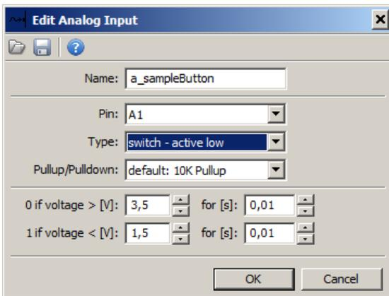
A configuration for a button connected to ground and to analogue input 1. The value **a\_sampleButton** will be 0 when the button is not pressed and 1 when it is.
