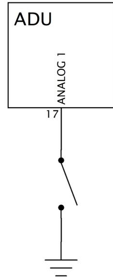
To preview the button state, open the **Analog inputs** panel, in which you will be able to track all **Analogue inputs**). The value of the button should equal 0 when not pressed and 1 when pressed.
