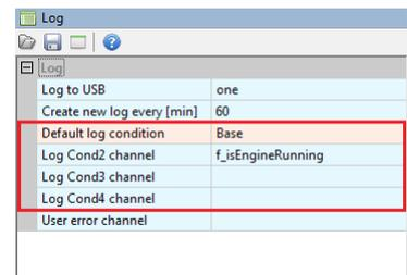
The screenshot shows a window titled 'Log' with a table of configuration options. The table has two columns: the left column lists the configuration item, and the right column shows its value. The 'Default log condition' row is highlighted with a red border.
