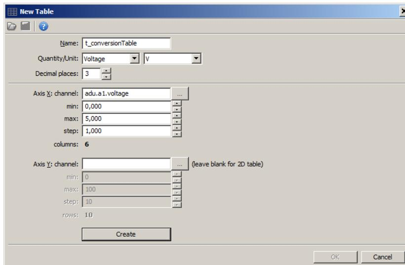
A **2D Table** will be created after pressing the **Create** button. The table should be modified so that 0V from the table is 5V, and for 5V - 0V.
