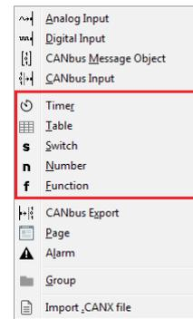
These elements are processed the same way as all elements in the ADU at 500 Hz (every 2 ms). These elements are processed in the listed above order (**Timers** first, then **Tables**, and so on).
