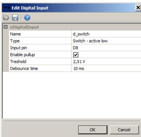
Configuration of the status read-out of the button connected to **Digital Input 8**. The button must connect the signal to ground. The **d\_switch** variable assumes a value of 0 when the button is not pressed and 1 when it is.
