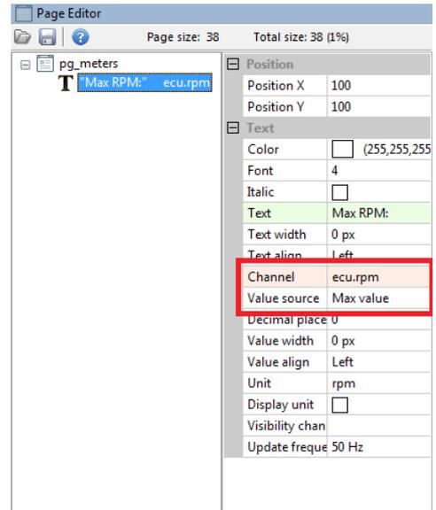
Just like the permanent meters, the min/max values of the ECU channels are recorded in the non-volatile memory of the device and remain in it even after the device is restarted.
