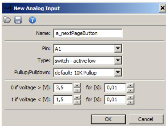
**Name** determines the name of the input that will be visible in the project. In the **Pin** field define the analogue input to which the button is connected (*Analog #1* in our case). Choose **Switch - active low** (which means that the button is activated at a low state). You also need to select a 10K pullup resistor.
