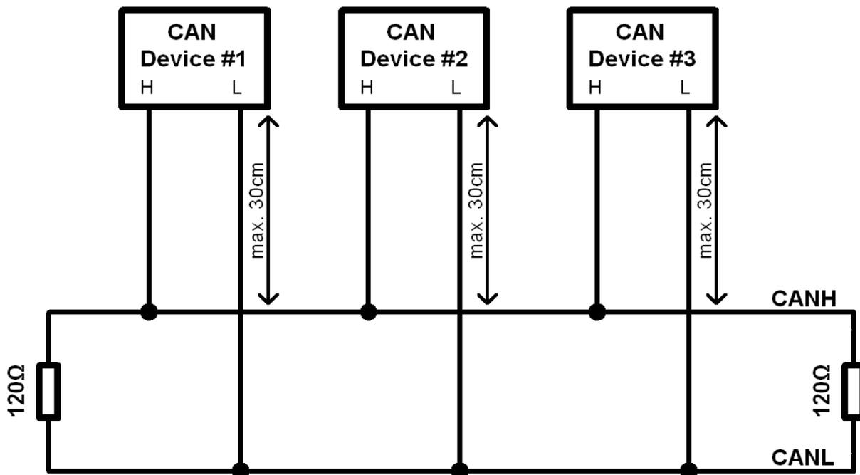
In automotive applications, typical data transmission speeds on the CAN bus are 1Mbps, 500 Kbps and 250 Kbps. Depending on the speed, the following conditions must be met:
