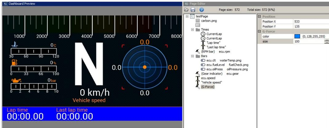
When using a GPS module, it is important that the user is able to see its status. To facilitate this, we will add a GPS status indicator. We will use two channels - *gps.status*, which shows us the GPS operation mode, and *gps.numSatellites* to show the number of satellites that the module is currently using.
