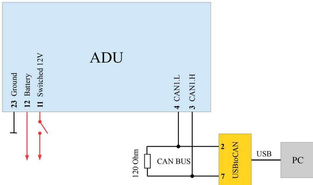
The above figure shows the minimum connections required to power the device and enable communication with a PC.
