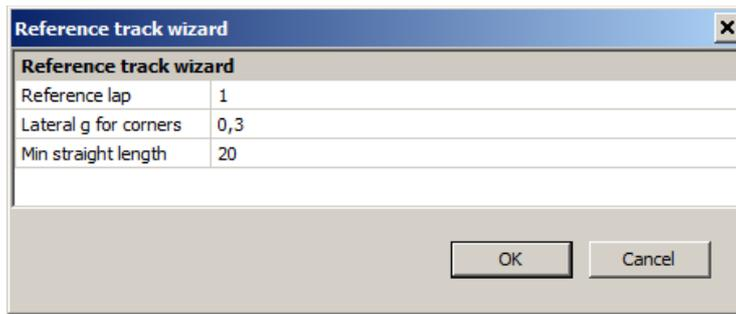
From the **Reference lap** field select the lap to be used for creating your reference track. As this lap changes in real time, the track contour will change, too. The **Lateral g for corners** parameter defines the lateral g-force above which a given track part is interpreted as a turn. The **Min straight length** parameter defines the minimum section of a track where the g-force was lower than **Lateral g for corners** for the distance to be considered a straight section.
