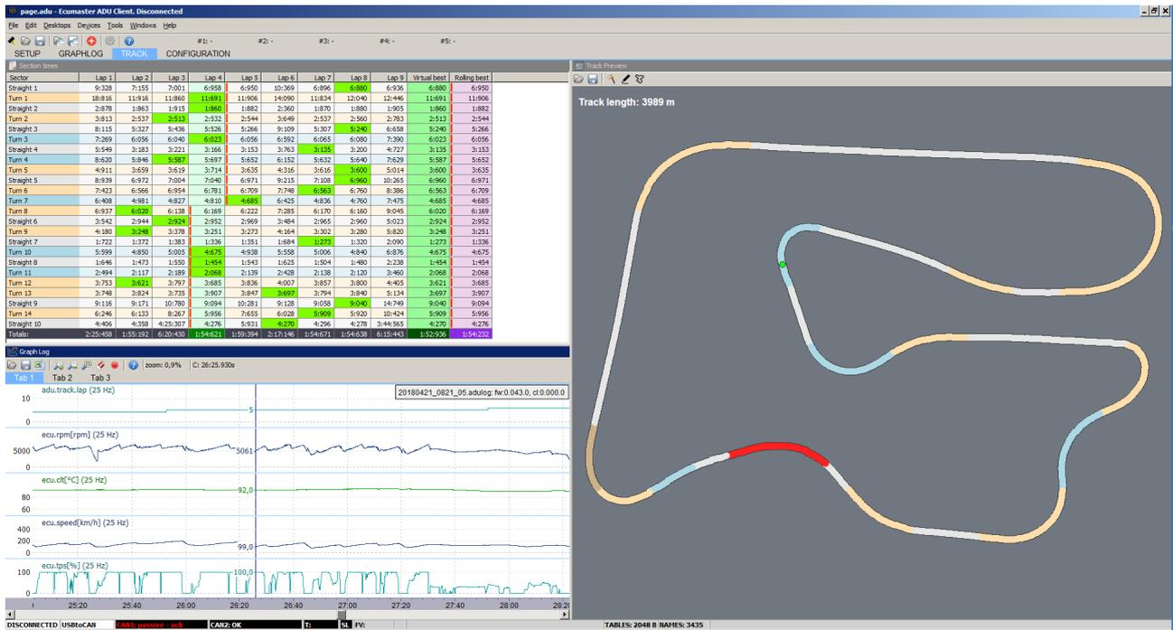
A green point on the reference track defines the car position for the position indicated in the log pane. This way, by moving along the log pane, you can see the set of parameters for particular car positions.
