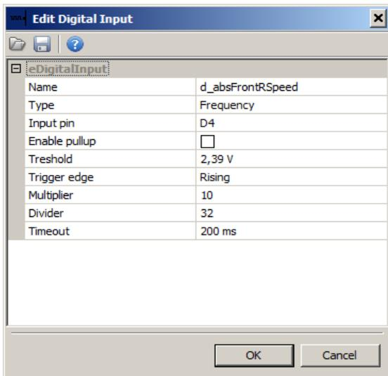
Configuration of a wheel speed read-out from an ABS sensor connected to **Digital Input 4**. The **d\_absFrontRSpeed** variable value equals the input frequency multiplied by 10 and divided by 32 (*multiplier, divider*).
