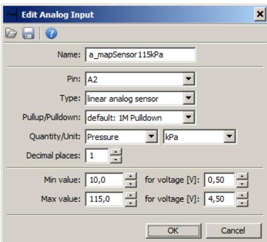
Configuration for a pressure sensor in the intake manifold (MAP) connected to analogue input 2. The value **a\_mapSensor115kPa** will assume values ranging from 10.0kPa to 115.0kPa
