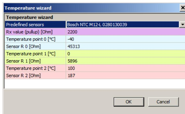
If the sensor characterization data is correct, a 2D map describing the sensor characteristics will be generated automatically:
