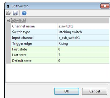
This element will operate as a counter. After each appearance of a **Trigger edge** in the **Input channel** the element will increase the value by 1. If the element already has a value equal to **Last state** and a **Trigger edge** appears, the value will “roll back” and assume the value of the **First state**.
