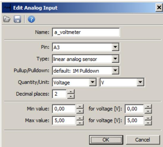
Configuration for measuring a voltage of 0-5V for a signal connected to analogue input 3.
