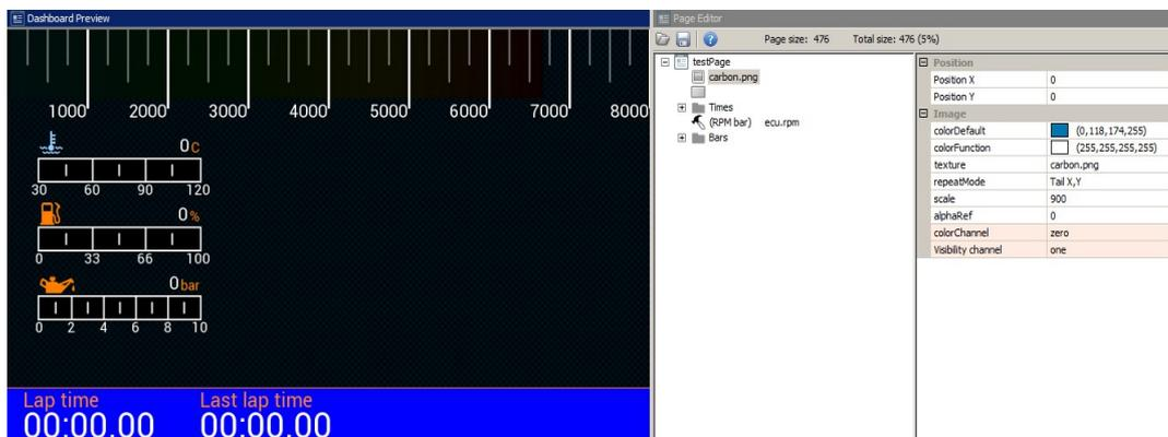
To insert an indicator for the current gear use *Gear indicator*. You should select a channel (*ecu.gear* in our case) and a font size. The indicator for the currently selected gear has a special font allowing to display large digits.
