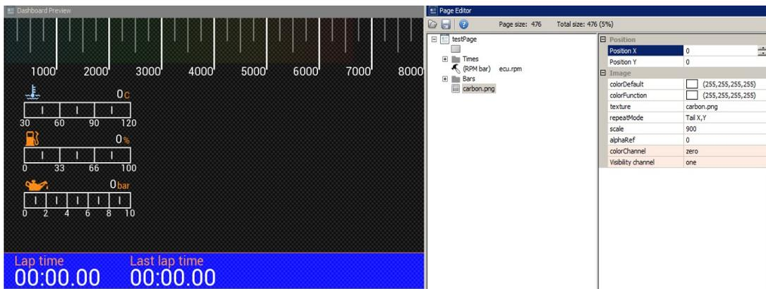
Note that our texture is displayed “over” the existing elements. To move it “underneath” we should rearrange it as the first element on the page. The order of application of elements is determined by their order on the list. To change their position on the list, select an element and move it by holding *ALT + up arrow* or *ALT + down arrow*. Let’s change the colour of our background to dark blue, too.
