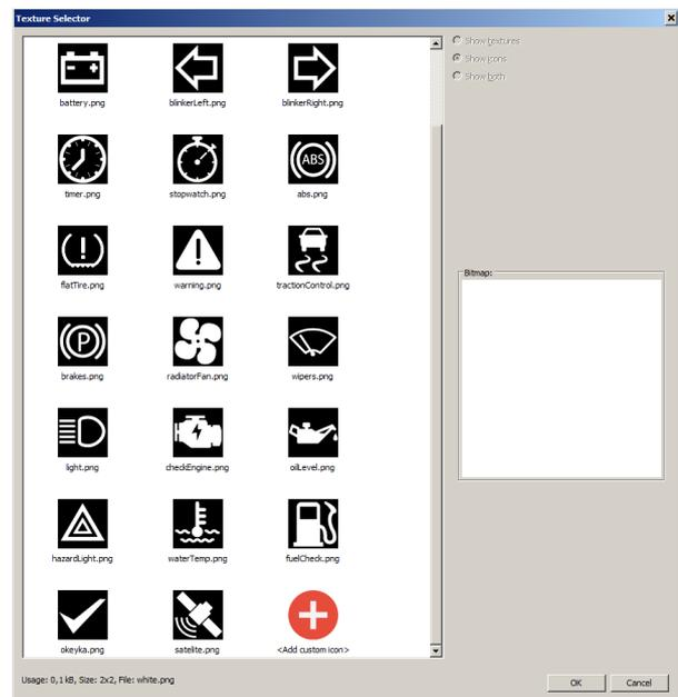
Next we will copy the created indicator twice in order to create a fuel level and oil pressure indicator. After copying, set their new position, select the appropriate icons and assign the appropriate channels in the **Channel** field. These will be *ecu.fuelLevel* for fuel level and *ecu.oilPress* for oil pressure, respectively. It is also worthwhile to group the indicators to facilitate their editing in the future. After copying the page your screen will look like the example below.
