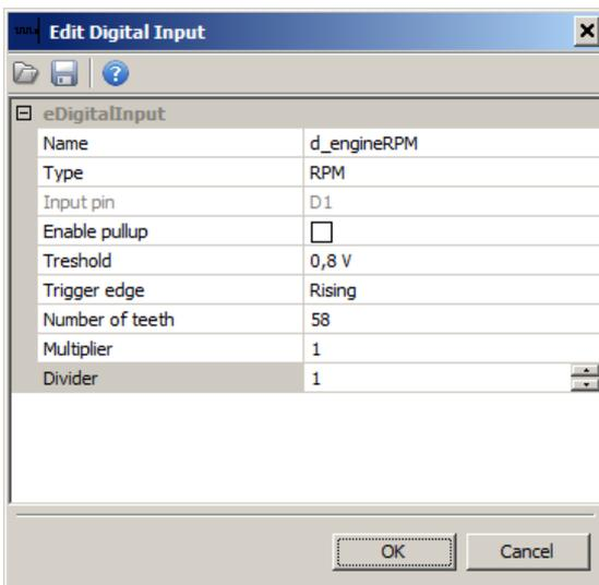
Engine speed (RPM) read-out configuration from an inductive crankshaft position sensor and a 60-2 trigger wheel. When using the engine speed read-out, the sensor must be connected to **Digital Input 1**
