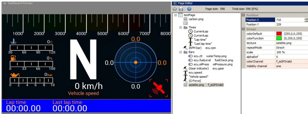
We will place two text fields over and under the icon. The upper field will indicate the number of satellites (*gps.numSatellites* channel), while the lower field will display the current GPS module status. For the *gps.status* channel, the text field will automatically transform the value into text (e.g. disconnected, gps 3D, etc.). We will group all elements of the indicators into a *GPS status* group.
